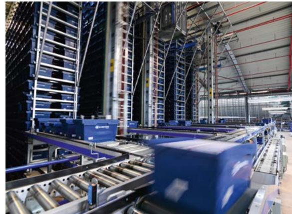
Bauerfeind has set up an automated small parts warehouse for the storage of numerous items, in which the products can be securely stored and transported in reusable boxes.
